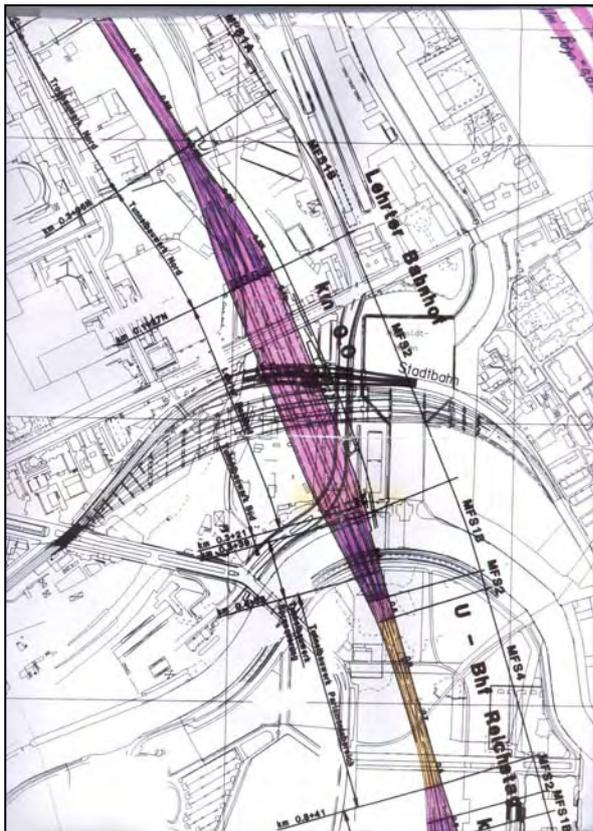
**Layout of the new Central Station of Berlin. The coloured North-South 8 station tracks underground and the 4 East-West station tracks and 2 S-Bahn tracks on viaduct.**
